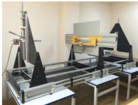
Figure 5. Space model of the experimental determination of orientation diagram.
