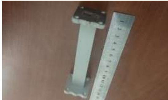
Figure 1. Space model of rectangular waveguide working in wave H_{10} .
